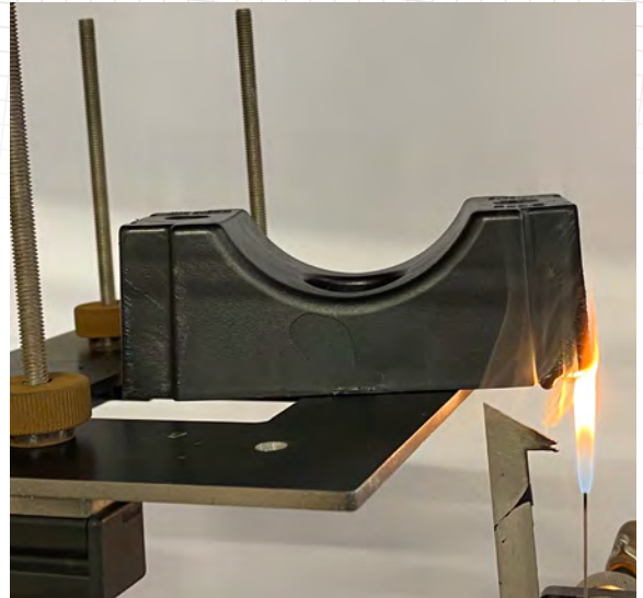
FLAME PROPAGATION TEST ON SOLUS NON-METALLIC CLEAT.
