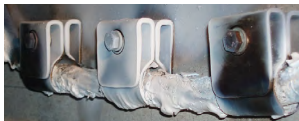
Phoenix clips have been fire tested in accordance with BS 589-1:2017
