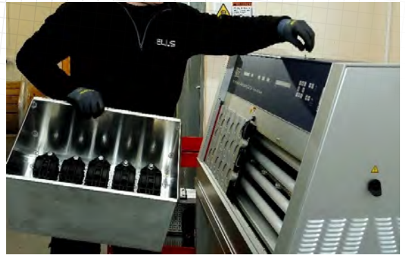
ELLIS' IN HOUSE UV WEATHERING TEST STATION
