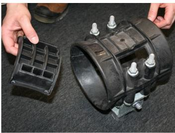
2) Using 24mm spanner/socket fix the cleat to the mounting structure. Tighten to a degree whereby the bracket is snug to the mounting but can still rotate on the base.
