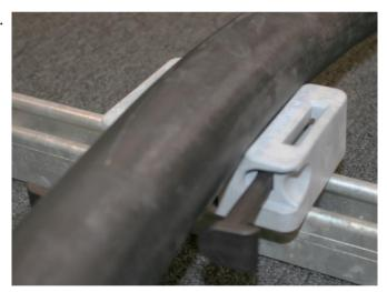
3) Insert the top part of the cleat into the base and apply firm downwards pressure. Whilst maintaining pressure on the top push the two keepers home to lock the cleat in place.
