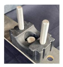
PLACE CLAMP ONTO STRUCTURE AND TIGHTEN THE CENTRAL M12 FIXING TO A TORQUE OF 10N.m.
