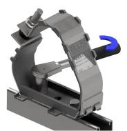
3) Tighten both bolts in the base of the cleat to the same torque value.
