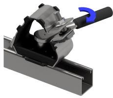
3) Tighten the M10 bolt in the base of the cleat.
