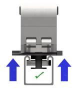
4) As the bolts are tightened the channel nuts will move up the twist foot base and grip onto the channel.
