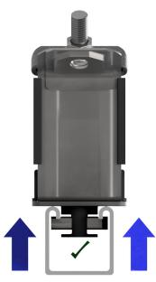
4) As the bolt is tightened the channel nut will move up the twist foot base and grip onto the channel.
