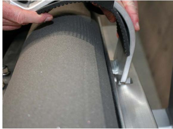
4) Close the strap onto the M12 fixings. Using a 19mm socket/spanner for the head of the set screws and an 18mm socket/spanner for the flange nuts, tighten the strap to an appropriate torque for the cable.
