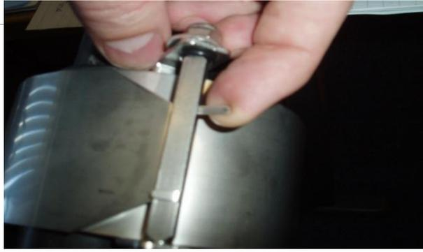
6) Using the 1/4" ratchet begin to turn the square end of the spindle clockwise, ensuring that the strap end remains in the spindle.
