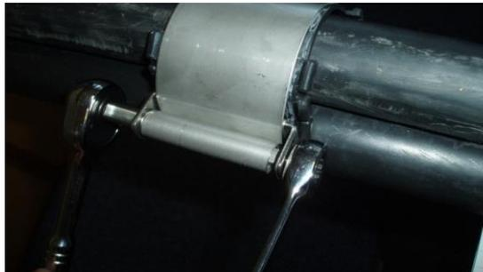
9) When correctly installed the square spindle should be in full location with the square hole in the frame.
