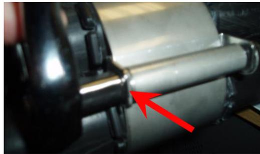
8) Using a 10mm spanner tighten the Nyloc nut at the other end of the spindle, thus drawing the spindle through the frame assembly.
