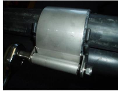
7) When the strap is tight around the cables, the square ratchet tool must be parallel to the top of the frame. This will ensure that the square spindle is 'in line' with the square holes in the frame.
