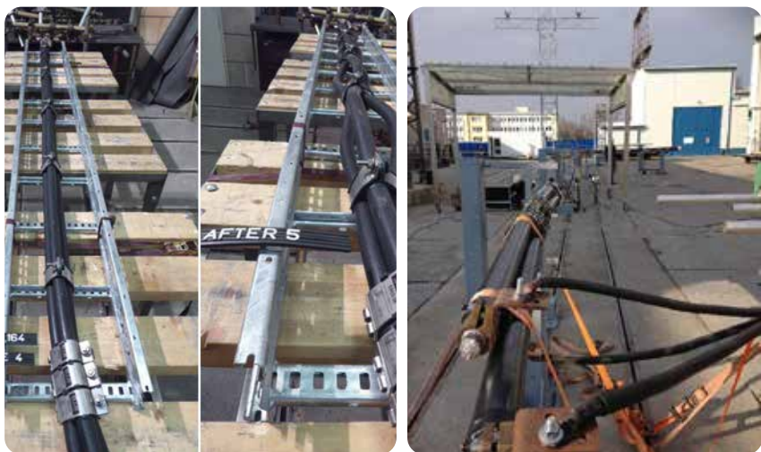
▲ Typical testing to IEC 61914 and bespoke testing of a HV test rig to a customer's specification.
