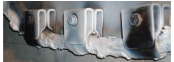
Phoenix clips have been fire tested in accordance with BS 8491 and BS 5839-1.
