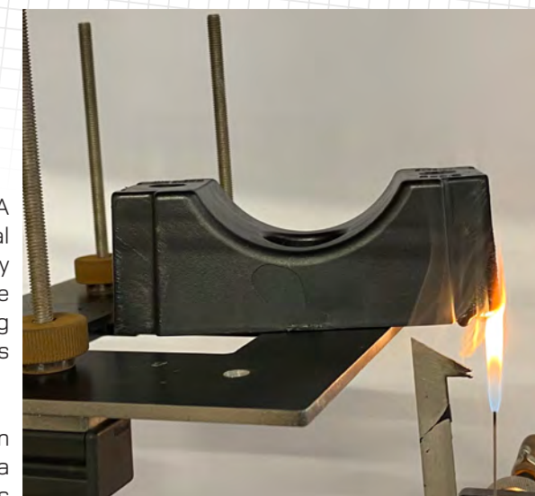
FLAME PROPAGATION TEST ON SOLUS NON-METALLIC CLEAT.
