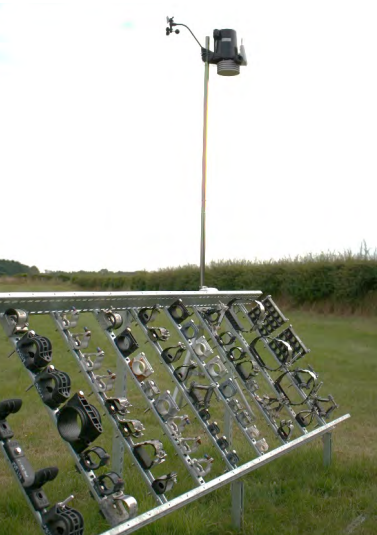
IN ADDITION TO THE CORROSION TESTING TO IEC 61914 ELLIS CARRIES OUT EXTENDED TESTING ON ITS OUTDOOR WEATHERING STATION.
